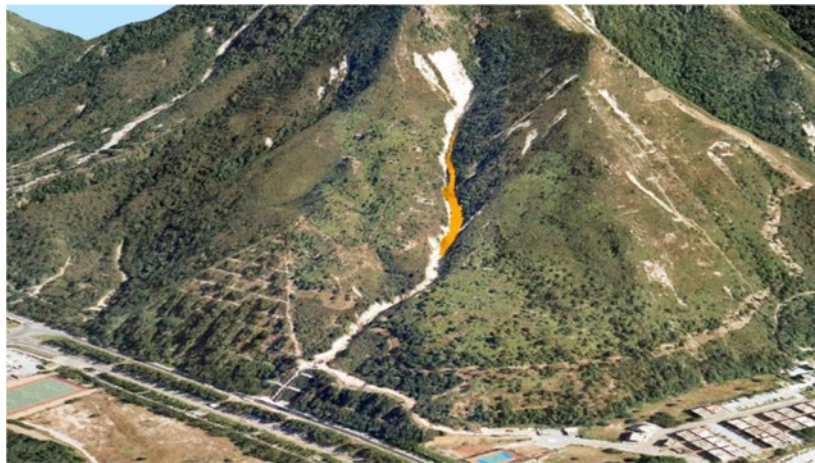
Figure 2: Simulated landslide motion in three-dimension using 3d-DMM (Version 2.0)
